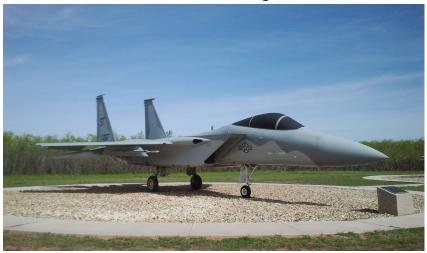
The F-15A Eagle is an all-weather fighter designed to gain and maintain air supremacy. First flown in 1972, the Eagle entered U.S. Air Force service in 1974. The Air Force ordered more than 350 "A" models for operational service. It was the first U.S. fighter with engine thrust greater than the basic weight of the aircraft, allowing it to accelerate while in a vertical climb.
