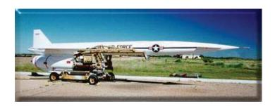
The Hound Dog was designed as a long range, stand-off air-to-ground strategic missile. It was carried in pairs beneath the wings of B-52 aircraft. Its development was initiated by the Air Force in 1957 during the early years of the cold war. It was designed to be carried on airborn alert B-52 aircraft to give them long range strike capability if needed. The first launch took place in 1959 when a Hound Dog was launched from a B-52G.
