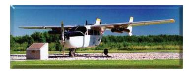
Originally this airplane was a Cessna 337 Super Skymaster. This unorthodox all-metal business aircraft resulted from several years of study by Cessna aimed at producing a twin-engine airplane that would be simple to fly, low in cost, safe and comfortable, while offering all the traditional advantages of two engines.
