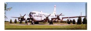
Bill Boeing's company built some very practical airplanes. Fatten the B-29's fuselage, use the same wings, tail and engines and you have a cargo plane. The prototype first flew in 1944 with the first production C-97A in 1949.
