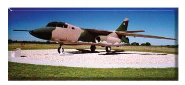
The B-66 was developed from the Navy A-3D "Skywarrior" for USAF use as a tactical light bomber and photo reconnaissance aircraft. The B-66 became operational in 1956, with production ending in 1958.
